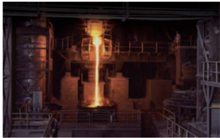
電気炉 Electric arc furnace
