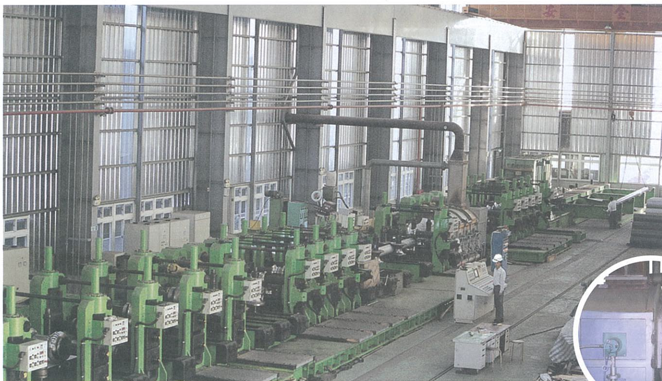
線上固溶化熱處理設備 on-line solution annealing furnace
